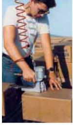
TOP P pneumatic. The pneumatic TOP P blind stapler and TOP EH onehanded blind stapler means that the operator has one hand free to shape the
