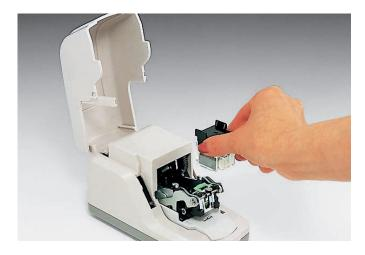
**HINGED COVER** The electronically secured cover can be opened safely for exchanging the flat staples cartridge.
